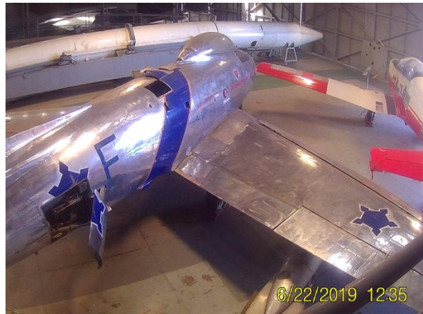
Preliminary polishing on the top surfaces after completion
