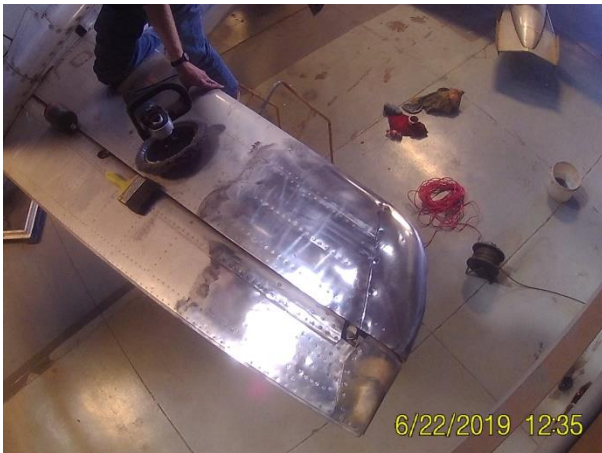
Preliminary polishing on the right elevator
