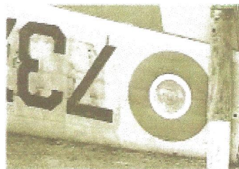
Standard "C" type roundel applied under the wing of Harvard 7370. An attempt has been made to modify the roundel in service with a small orange centre and the rest filled in with white. The roundel has faded in the sun to its original proportions.
