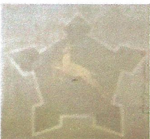
This 'low viz' castle is a standard one which has been overpainted with a light coating of grey on a Mirage F1CZ.
