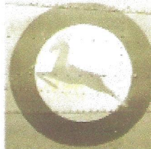
Standard Springbok Roundel as applied to a Harvard. Colours are Light Orange Springbok and Aircraft Blue outer Ring. Note how rear foot of Springbok cuts into Blue ring.
