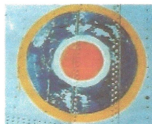
The C1 roundel applied at Harvard early post war was in bright colours using Ultramarine instead of the usual Dull Blue.
