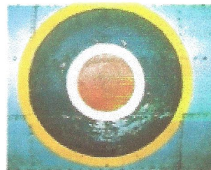
Standard proportion Type C1 roundel on a Spitfire with yellow outer ring some width as white inner ring. Standard dull blue has been used.
